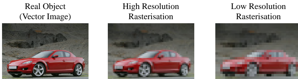
Figure 8: Demonstration of the rasterisation of a real object with high and low resolutions. (Although the original image of the real object is actually a raster image, its resolution is sufficiently large to avoid raster artefacts and it serves as a view from an observer for this demonstration).
